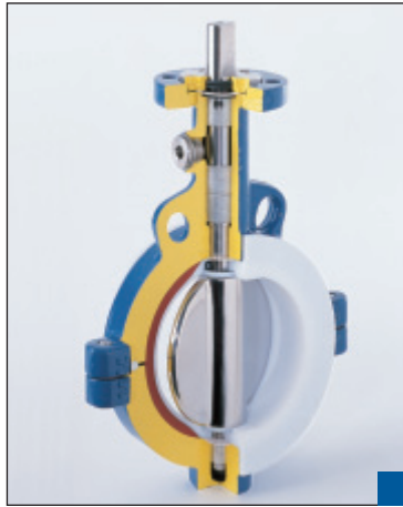
TA-Luft sealing on the top flange. GAR-SEAL valves fulfil the high demands regarding tightness against atmosphere. A leakage control device can be integrated upon request.
